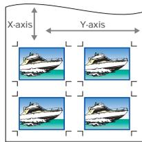
Multiple imposition data sequentially positioned in the X and Y axis directions are individually corrected and cut correctly.
